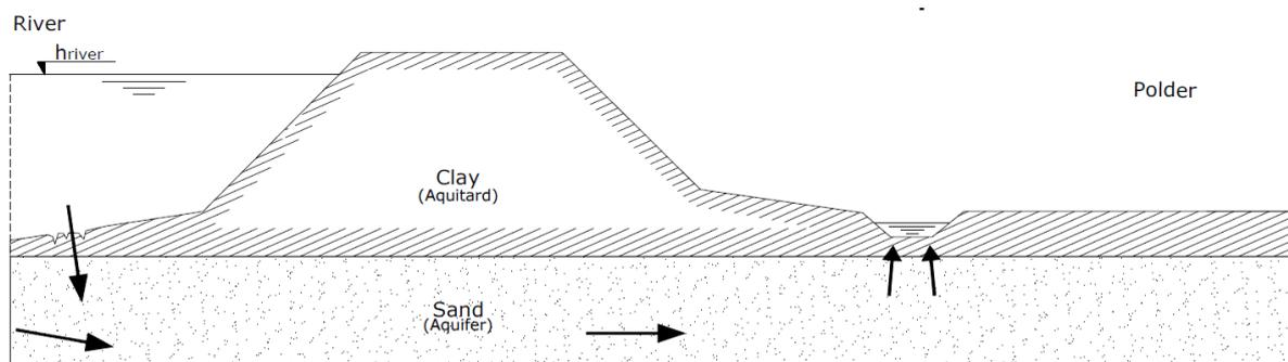
Figure 3.6: Schematic problem Pipingontspanner
