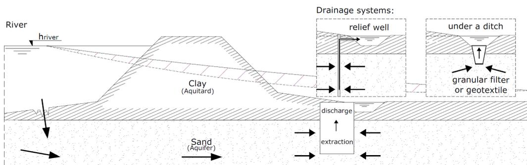
Figure 1.6: Schematic representation of a relief well and gravel filter (Niemeijer et al., 2017)
