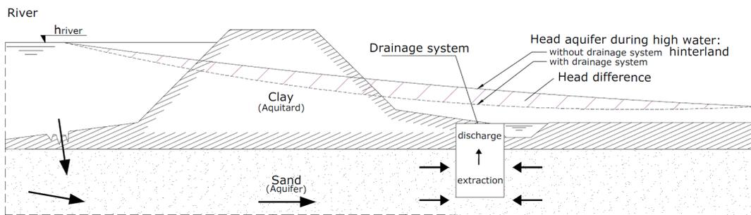
Figure 1.5: Schematic representation of a drainage systems near a dyke during high water levels (Niemeijer et al., 2017)
