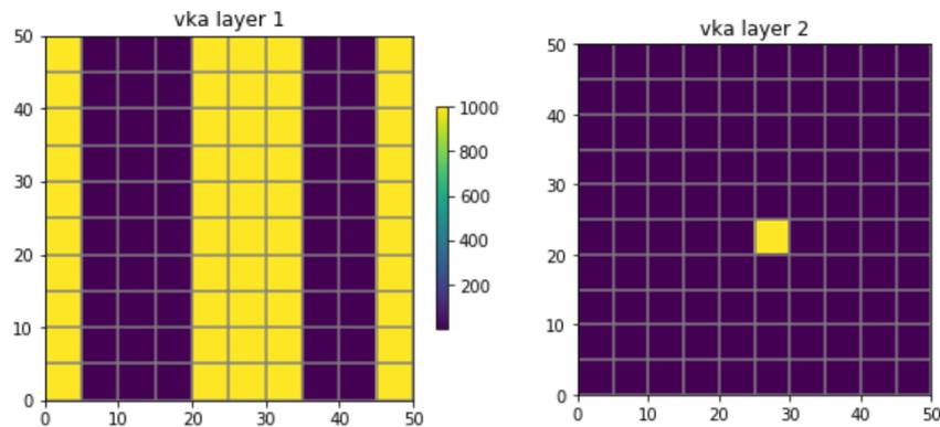
Figure 2.10: Vertical hydraulic conductivity of the well cell, layer 1 and layer 2
