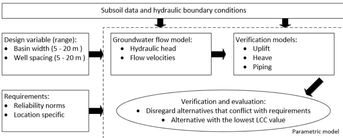
Figure 3.9: Overview parametric design
