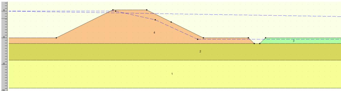
Figure 4.11: Input D-Geo Stability Base scenario
