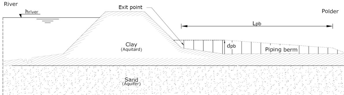
Figure 5.18: Overview Piping berm design
