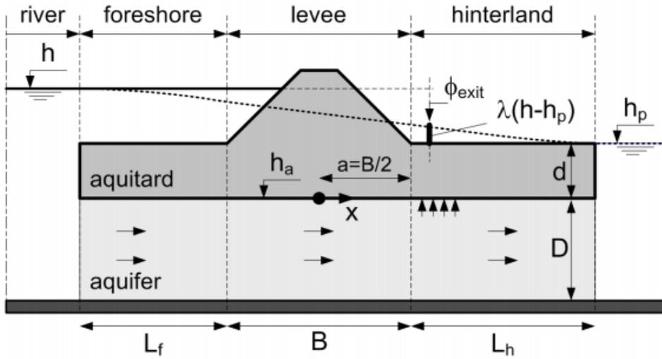
Figure 1.4: Definitions relevant for limit state (Schweckendiek, 2014)
