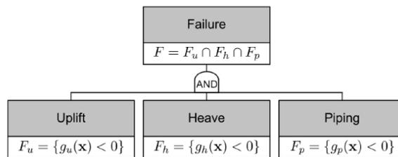
Figure 1.3: Fault tree mechanism piping (Backward internal erosion) (Schweckendiek, 2014)
