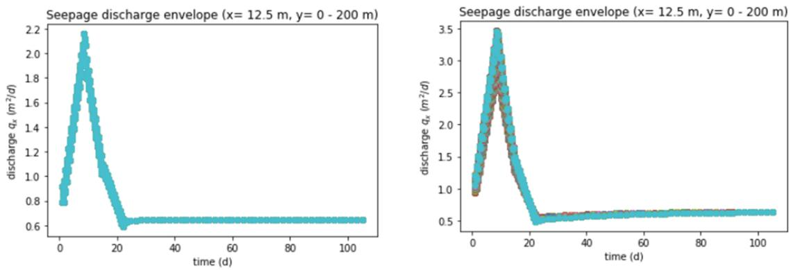
Seepage discharge from the river (base (l) and Pipingontspanner situation (r))
