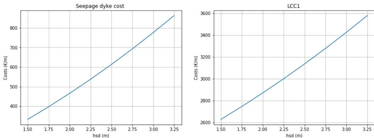
Figure 5.7: Seepage dyke costs for varying dyke height ( $h_{sd}$ )
