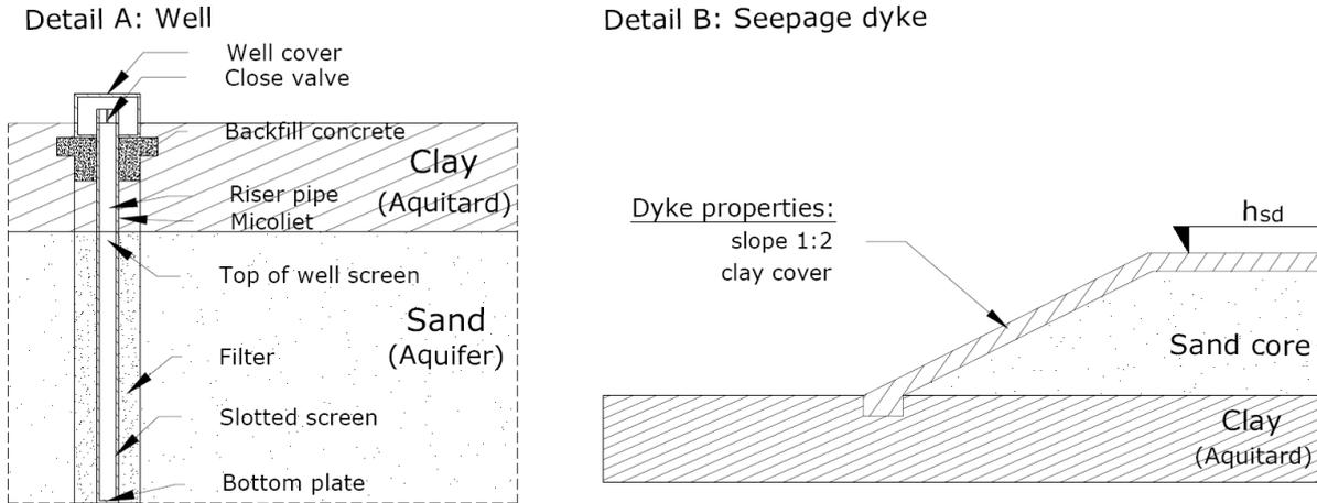
Figure 5.3: Pipingontspanner general design details
