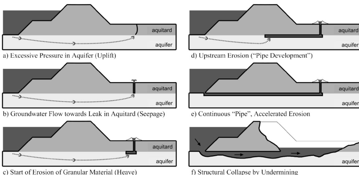
Figure 1.2: Description of the piping process (backward internal erosion) (Schweckendiek, 2014)
