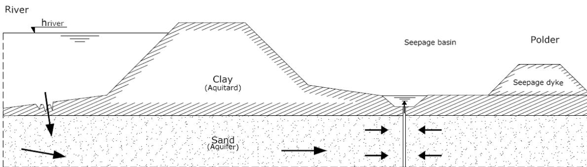
Figure 2.3: Schematisation of the Pipingontspanner with a relief well
