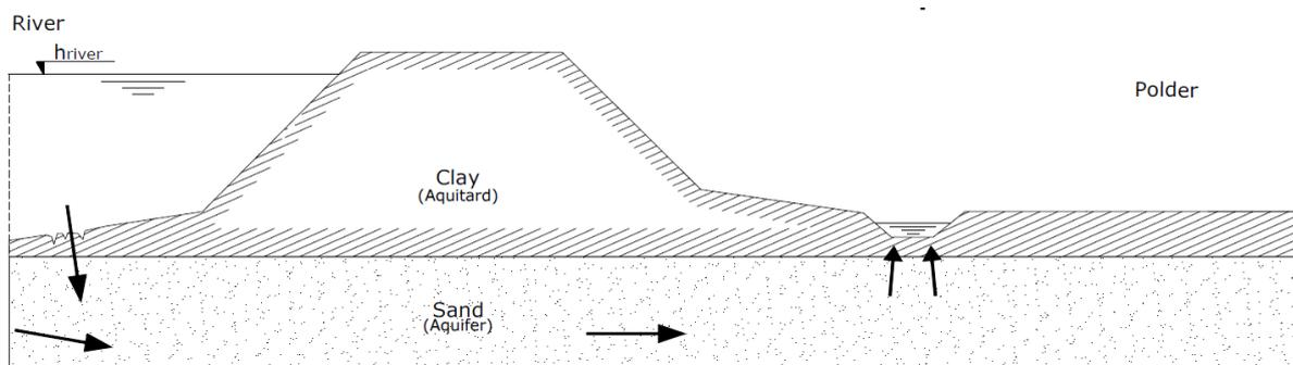
Figure 2.1: Schematisation of seepage flow under a dyke (Technische Adviescommissie Waterkeringen, 1993)
