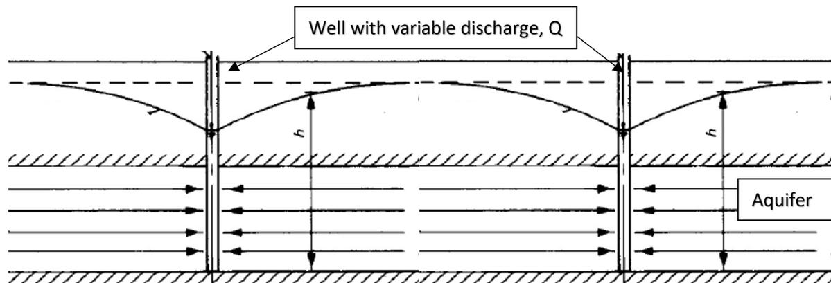
Figure 1.12: Schematic representation of a relief well along the dyke length Y-Z plane (Adapted (USACE, 1986))
