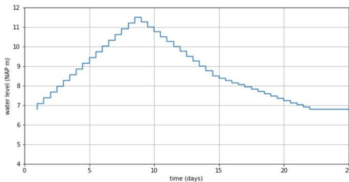
River boundary: schematisation: design flood wave (River Waal, Tiel)
