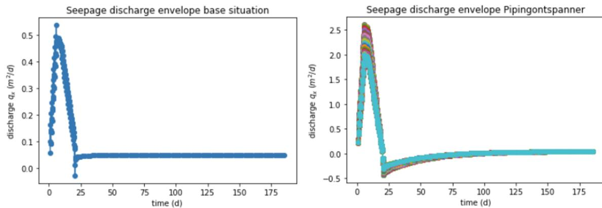
Figure A.2: Seepage discharge envelope base and Pipingontspanner situation ( $x = 12.5$  m,  $y = 0 - 50$  m)
