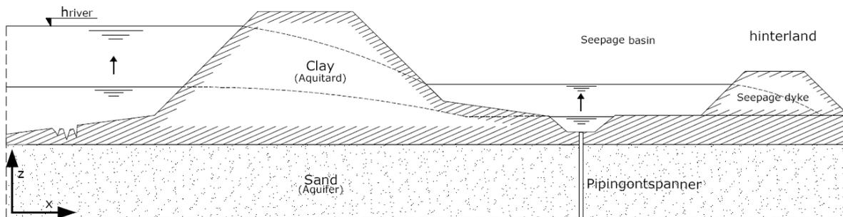
Figure 1.11: Schematic representation Pipingontspanner cross-section X-Z plane
