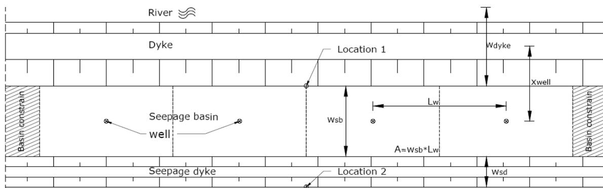
Figure 5.15: Overview Pipingontspanner design variables
