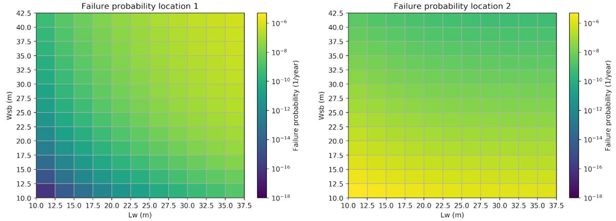
Figure 5.16: Failure probability location 1 (inner dyke berm  $x=52$  m) and 2 (behind seepage dyke  $x = 52 + w_{sb} + w_{sd}$ )
