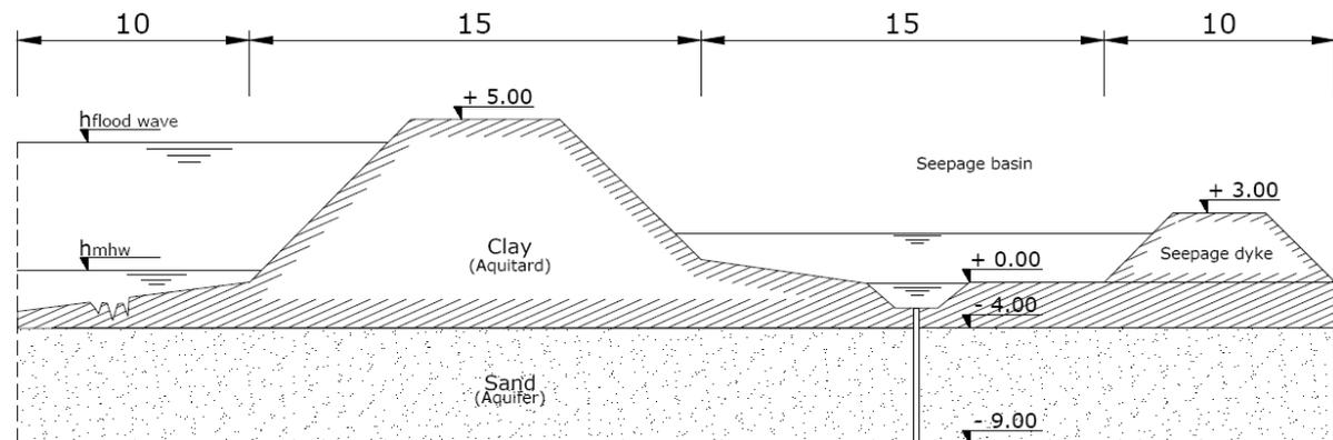
Figure 2.4: Principle sketch for flow mechanism
