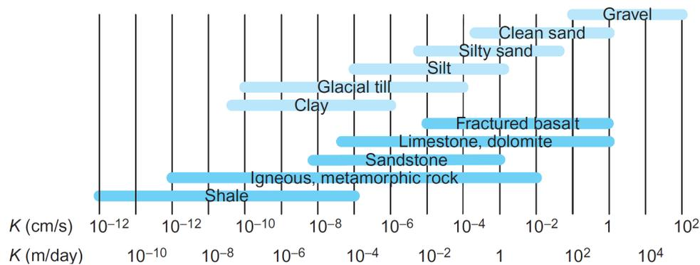
Figure 2.2: Typical values of hydraulic conductivity based on experiments (Fitts, 2002)
