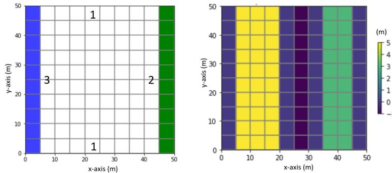
Figure 2.8: Boundary conditions on the grid (x,y)
