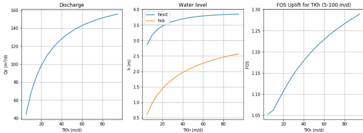
Figure 4.4: Sensitivity transmissivity aquifer
