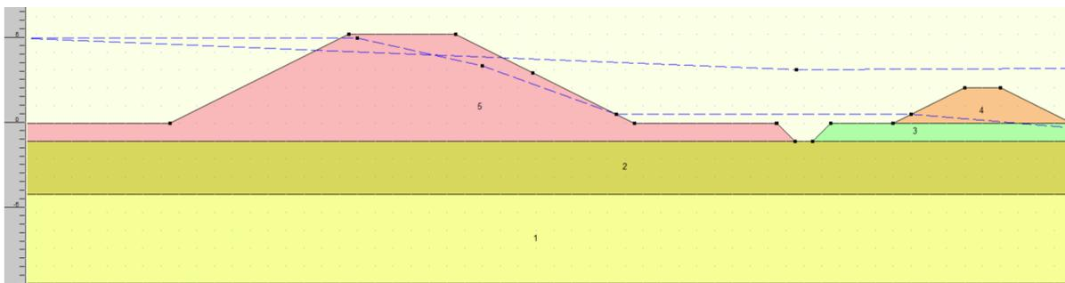
Figure 4.12: Input D-Geo Stability Pipingontspanner scenario
