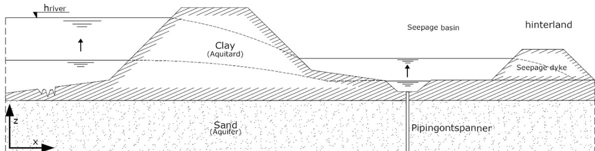
Figure 1.7: Principle cross-section of the Pipingontspanner
