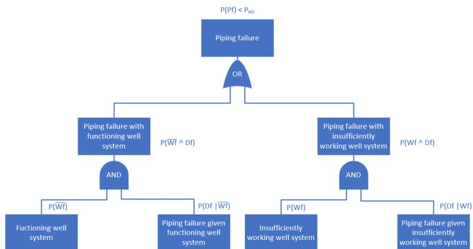
Figure 3.2: Fault tree Pipingontspanner
