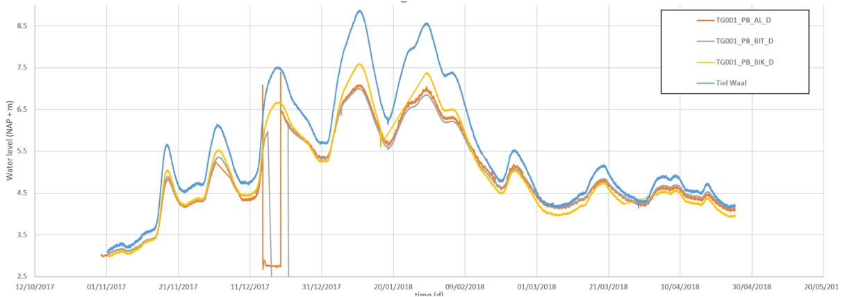
Figure 5.10: Monitoring wells aquifer on cross section (Waterschap Rivierenland, 2018)
