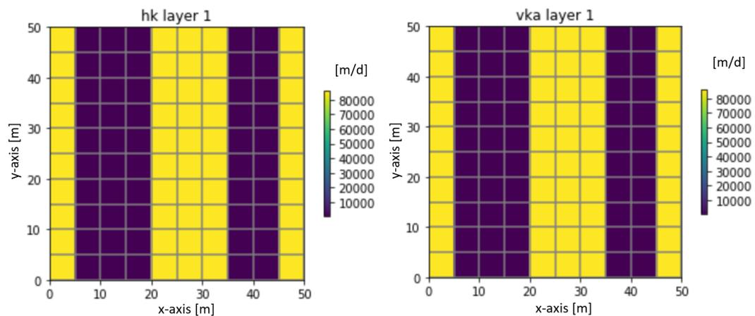
Figure 2.7: Hydraulic conductivity horizontal and vertical, left and right respectively
