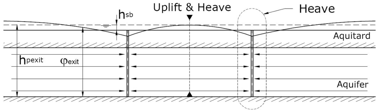
Figure 3.3: Assessment location Uplift and Heave mechanisms
