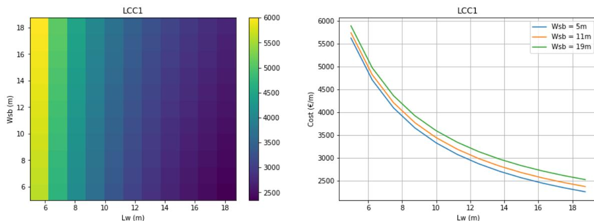
Figure 5.5: Life Cycle Costs for varying design variables ( $L_w$  and  $w_{sb}$ )
