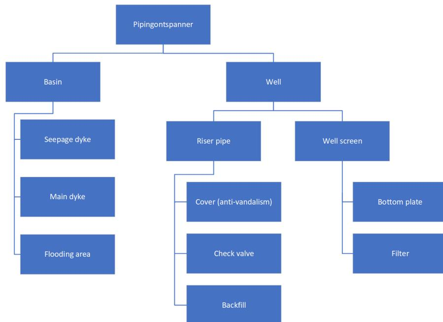
Figure B.1: Object tree Pipingontspanner
