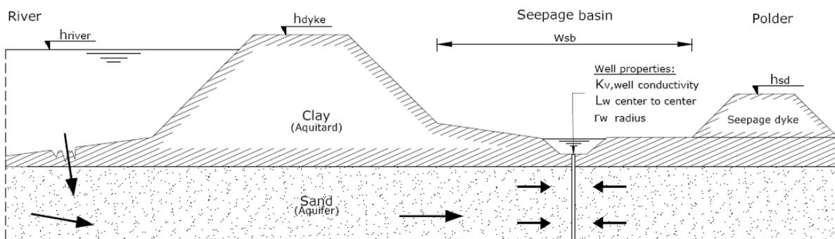
Figure 3.7: Schematic Pipingontspanner variables
