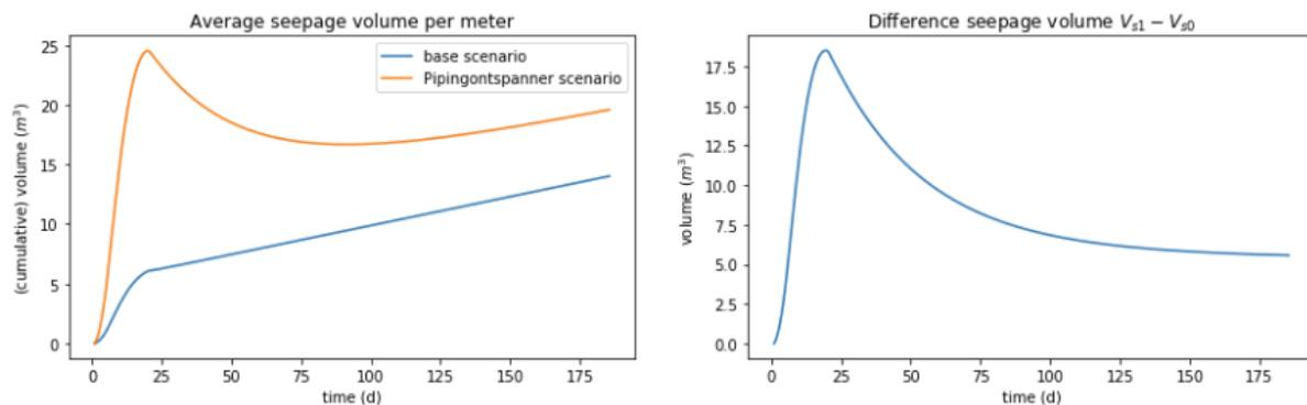
Figure A.3: Seepage volume base and Pipingontspanner situation ( $x = 12.5$  m,  $y = 0 - 50$  m)
