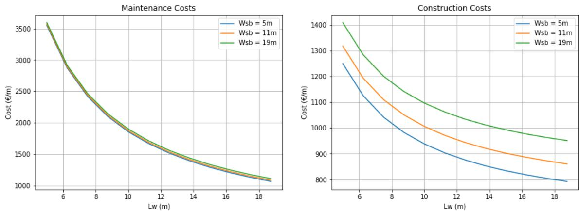
Figure 5.6: Maintenance and construction costs for varying design variables ( $L_w$  and  $w_{sb}$ )
