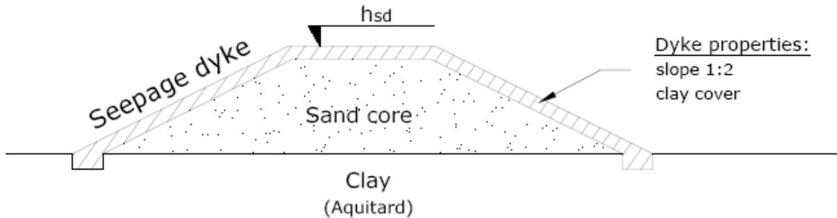
Figure B.2: Design seepage dyke
