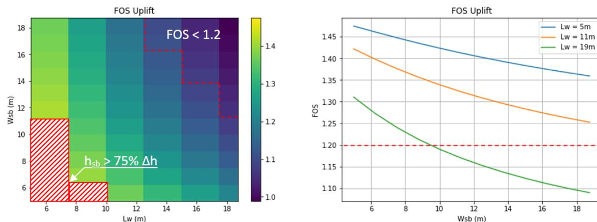
Figure 4.10: Operating conditions:  $w_{sb}$  &  $L_w$
