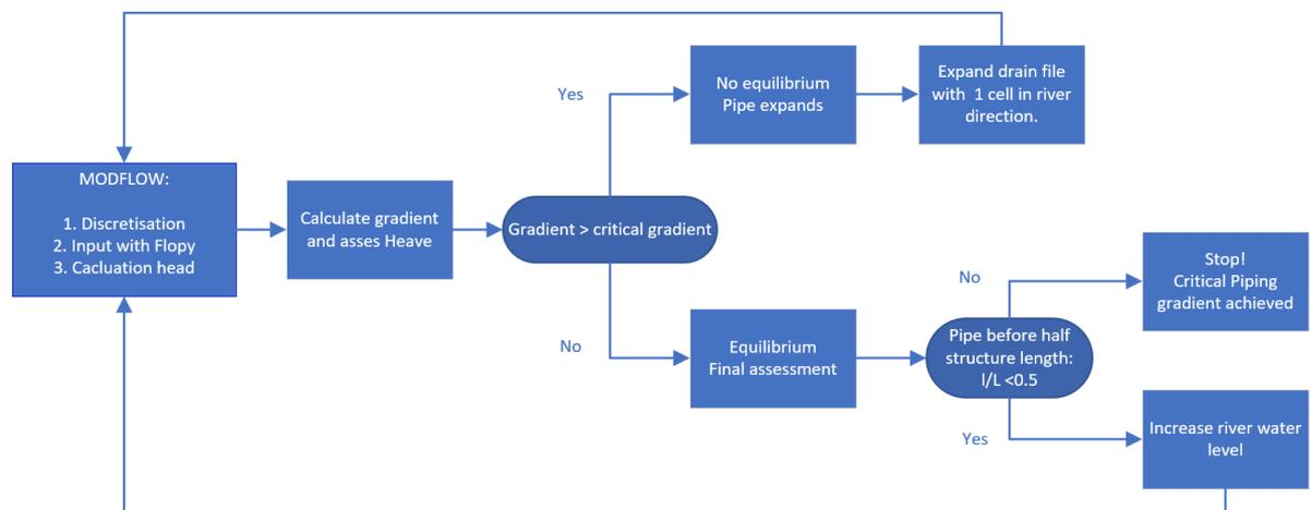
Figure 3.4: Approach to implementing Pipe development (adapted schematic (Schoonen and Mols, 2015))
