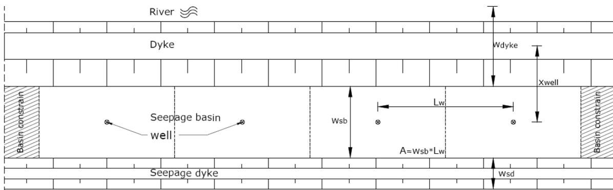
Figure 3.8: Overview Pipingontspanner design variables
