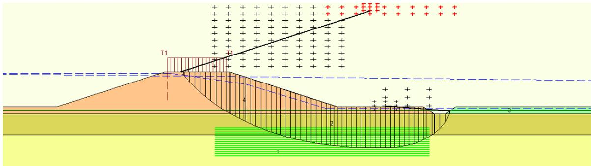
Figure 4.13: Result stability Uplift - Van Base scenario
