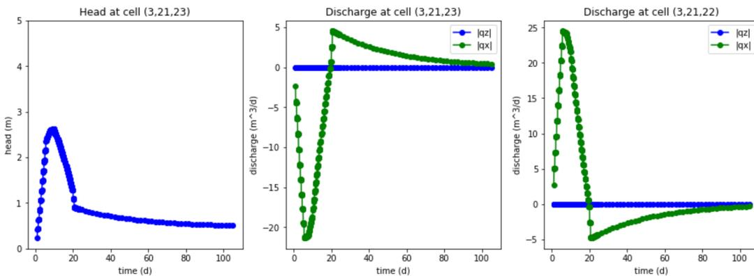
Detail D: Head and discharge in layer 3
