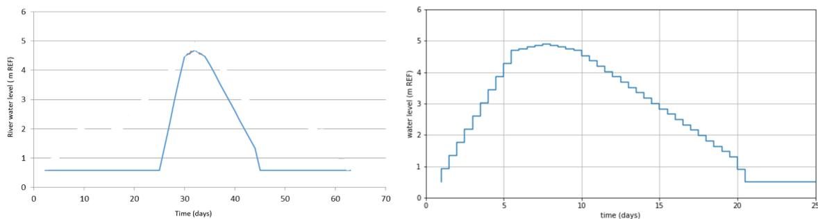
Figure 2.9: Flood wave example and schematisation, left and right respectively
