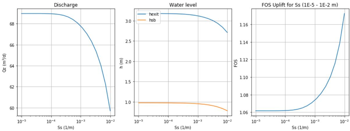
Figure 4.6: Sensitivity specific storage factor
