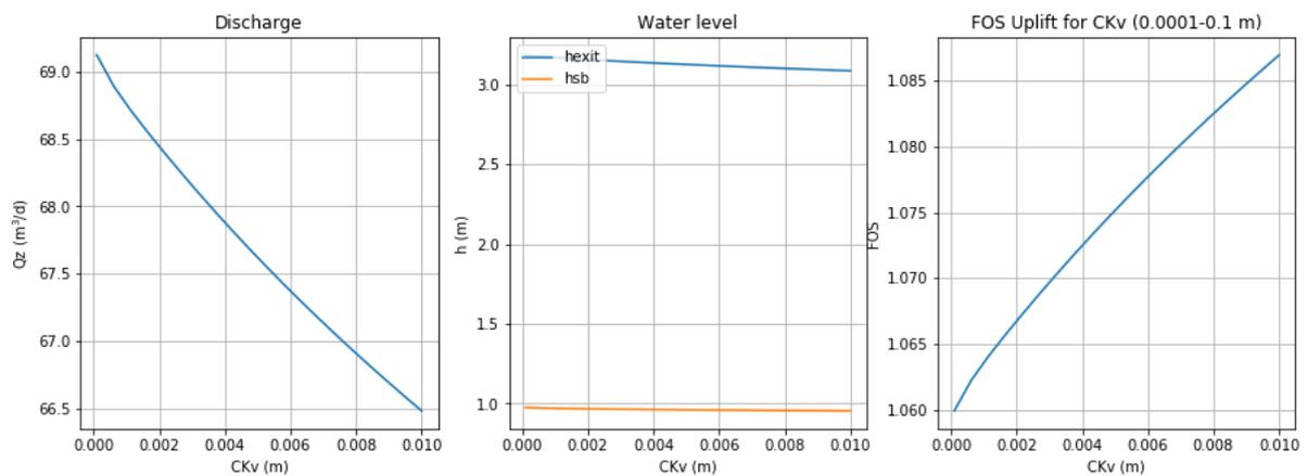
Figure 4.5: Sensitivity hydraulic resistance aquitard
