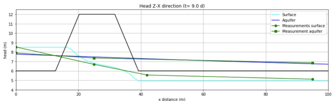
Figure 5.13: Calibrated Groundwater flow model with data monitoring wells
