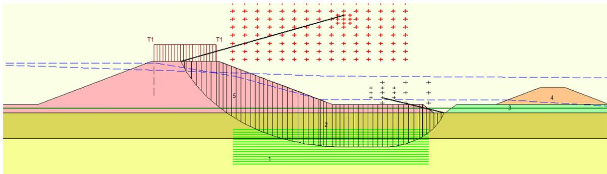
Figure 4.14: Result stability Uplift - Van Pipingontspanner scenario
