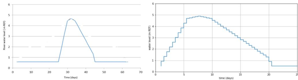
River boundary: schematisation: example flood wave (River lek, langerak) and Modflow input
