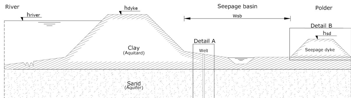
Figure 5.2: Pipingontspanner general design
