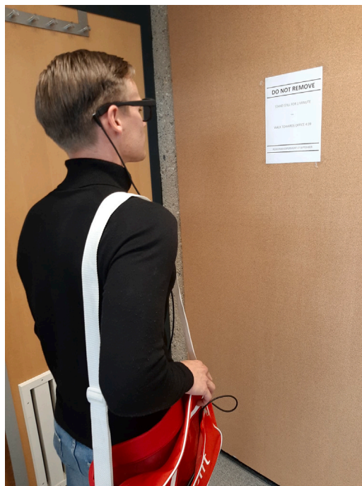
Fig. 2. An example of a participant equipped with the eye-tracking glasses connected to a mobile phone located in the red shoulder bag.
