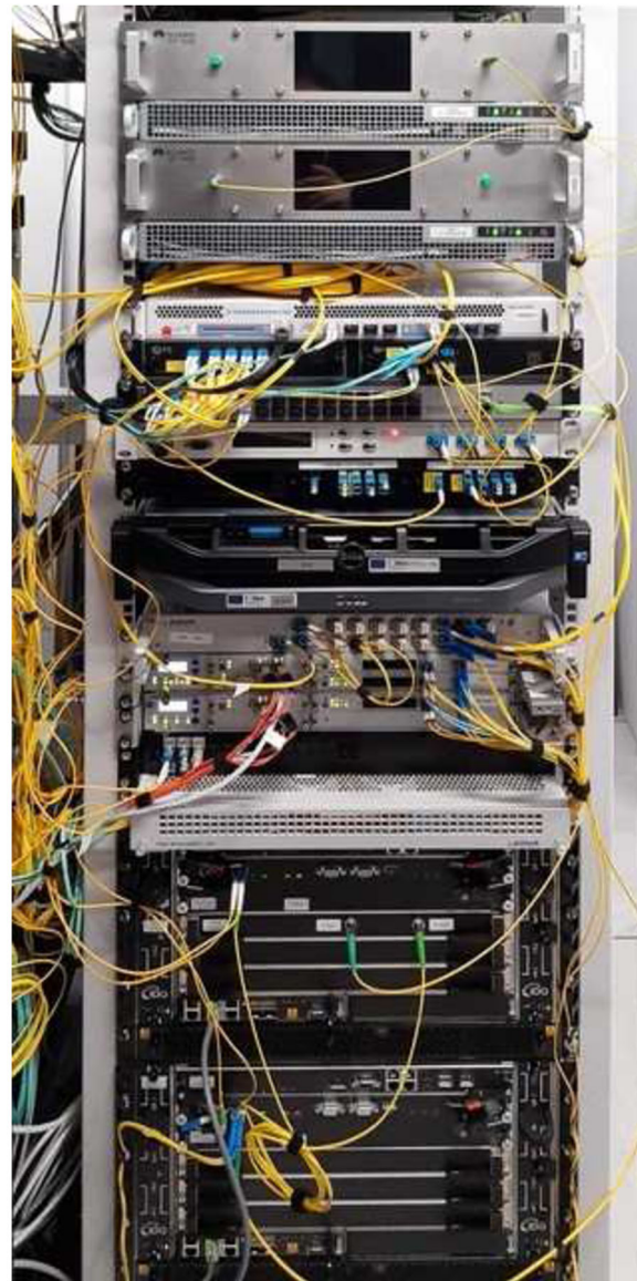
Figure 4 One of the central nodes in the Madrid QKD testbed, showing several QKD systems by different vendors in an equipment rack (Courtesy Vicente Martín, UPM Madrid)
