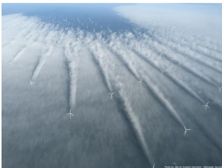
**Figure 2.1:** Horns Rev, North Sea, Denmark- Low-hanging fog leads to a picturesque visualization of the wake generated by a wind turbine - *photo by Bel Air Aviation Denmark-Helicopter Services. January 26th, 2016*
