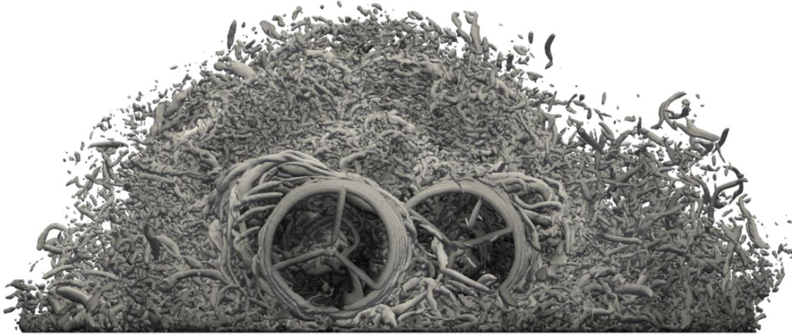
**Figure 6.3:** A Q-criterion iso-surface visualizing the turbulence generated in the wake as well as the helical tip vortices in L2 8m/s case. A value of  $Q_{crit} = 0.02s^{-2}$  is used as the threshold.
