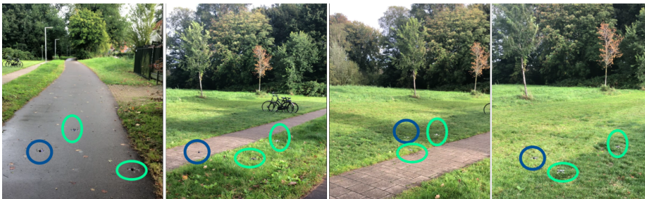
Figure 3.17: Outdoor formation flights of three Crazyflies. The leader is controlled manually for safety, while two followers fly fully autonomously purely based on onboard relative localization. The environments consist of winds, grass and sunlight. The full experiment can be found in the video.
