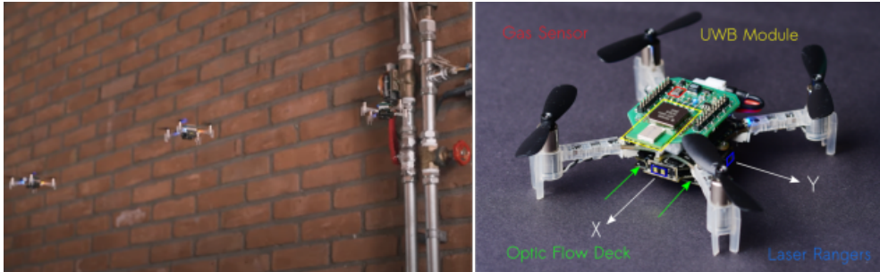
Figure 6.1: Example application of the proposed tiny aerial swarms for a gas-seeking task [1]. It proposes a bug algorithm for an autonomous swarm of quadrotors, to localize a gas source in cluttered environments.
