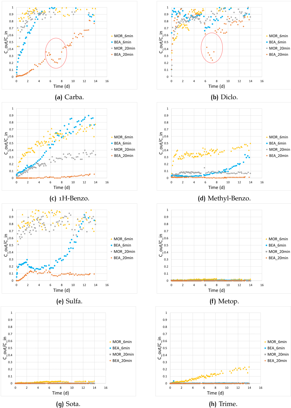
Figure 3.11: Breakthrough curves of OMPs in demi-water by BEA and MOR columns at EBCT of 6 min and 20 min
