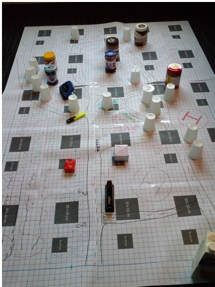
Figure 4.14: First set-up of the map, a grid used for overlap measurement, with objects for a three-dimensional simulation.
