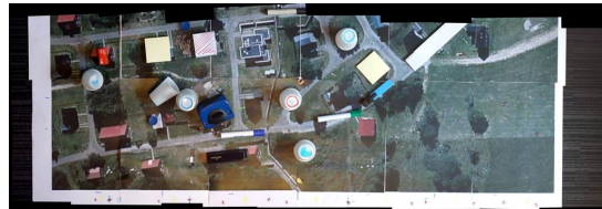
Figure 4.19: The stitched photomap consisting of photos of the second map, overlapping by 30 percent.
