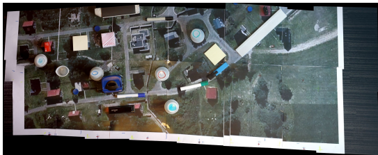
Figure 4.18: The stitched photomap consisting of photos of the second map, overlapping by 20 percent.
