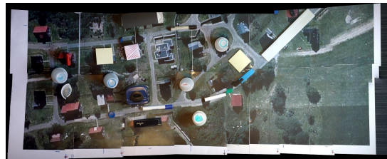
Figure 4.17: The stitched photomap consisting of photos of the second map, overlapping by 10 percent.
