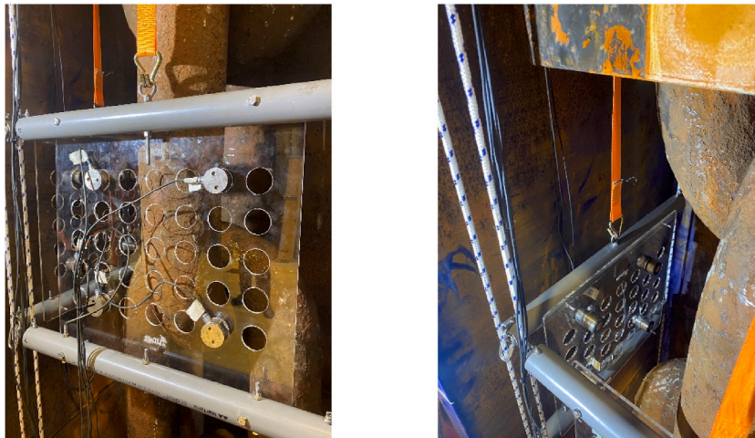
Fig. 4. Perpendicular movable arrays of AE transducers.
