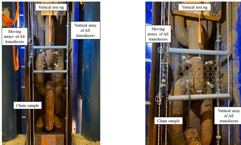
Fig. 3. Instrumented test rig (left) and non-contact sensors deployment in the test rig (right).
