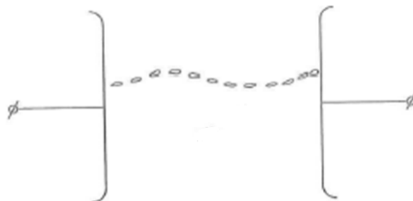
Figure 3.12: Particles bridging the electrodes [27]
