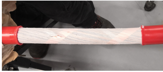
(a) Water Blocking Sheath.
