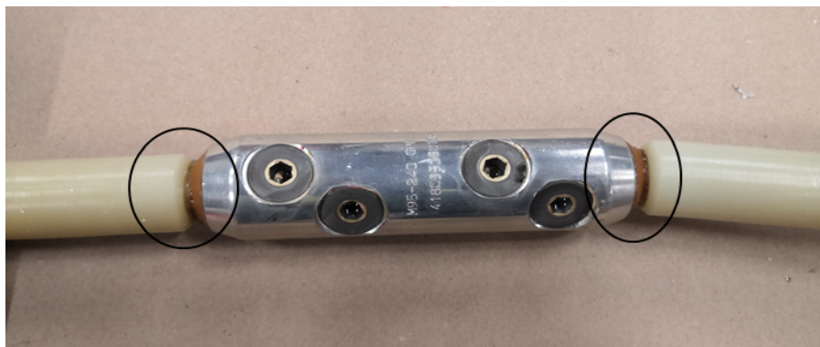
Figure 6.25: Examining the bolted connector present inside the joint housing.
