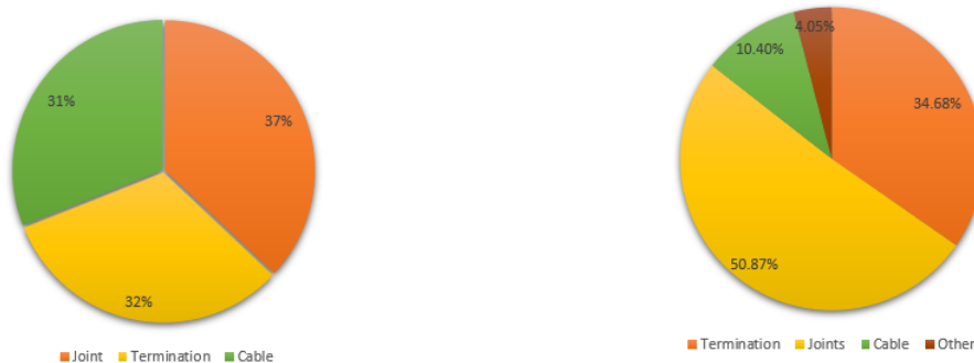
(b) Failure Location in the 110-220 kV cable systems as per the data collected by China Southern Power Grid.
