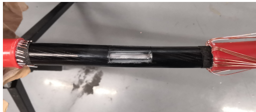
(b) Aluminium Conductor.
