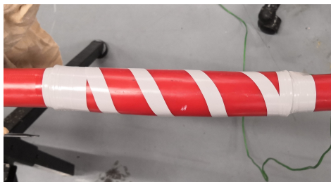
Figure 6.17: Rebuilt Cable after Placing the Thermocouple.
