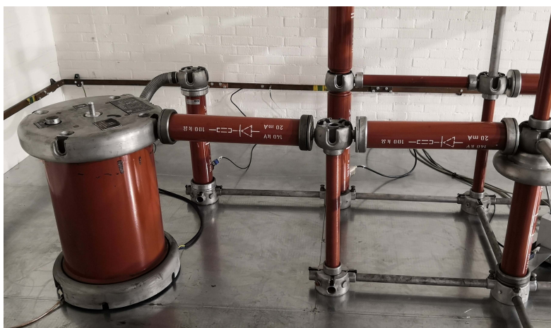
Figure 6.12: Diode Arrangement to Obtain Desired Polarity.
