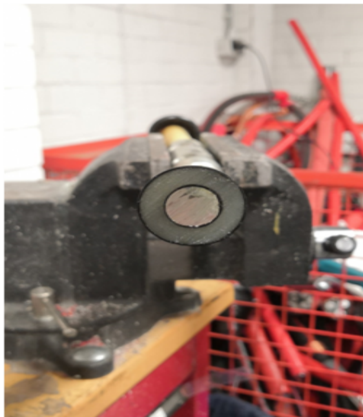
(a) Cable dissected at location 3 inside the joint.
