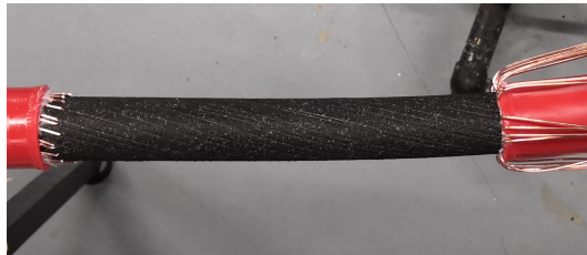
(c) Water Blocking Sheath.
