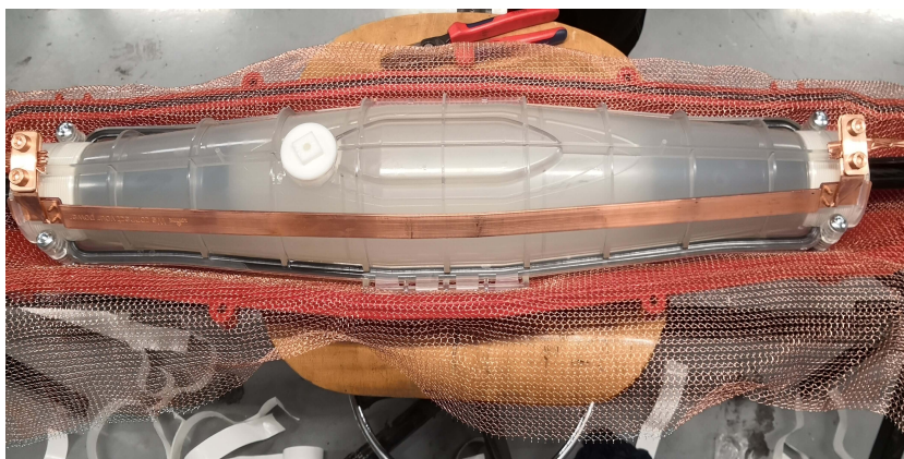
Figure 6.8: Inner shell covered with Copper mesh.
