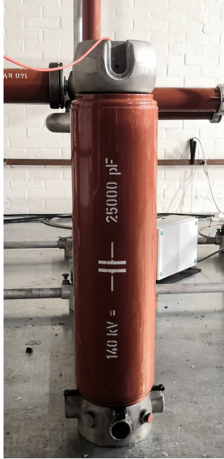
Figure 6.13: Capacitor for smoothening the DC output voltage.
