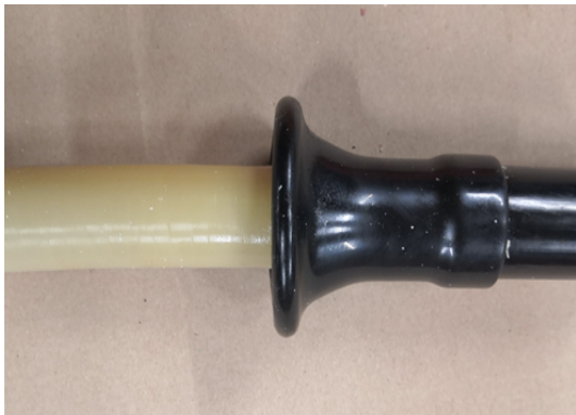
(a) Geometric field grading as part of the joint.
