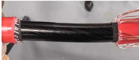
(a) Semi-conductive layer over the XLPE.
