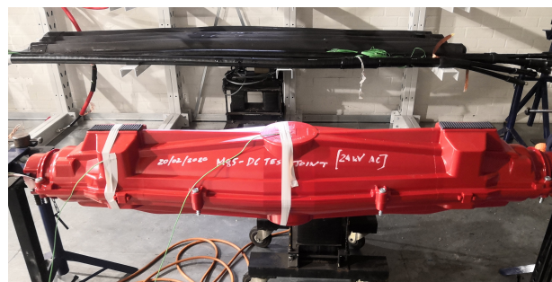
(a) Thermocouple at the centre and the beginning of the joint body.
