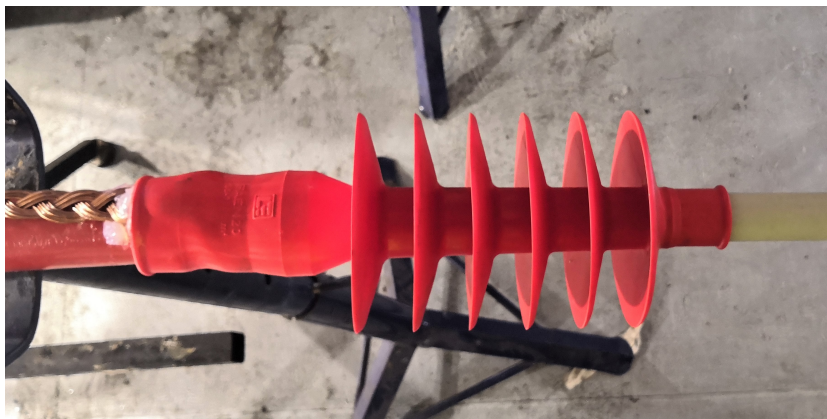
Figure 6.10: Termination with geometric field control.
