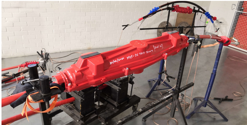
Figure 6.9: M85 Joint Built for Test.
