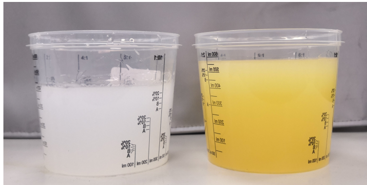
Figure 6.22: Discoloration of liquid Lovisil post testing.
