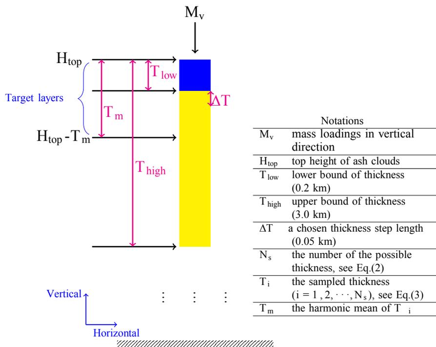
**Figure 2.** Illustration of the satellite observational operator (SOO).
