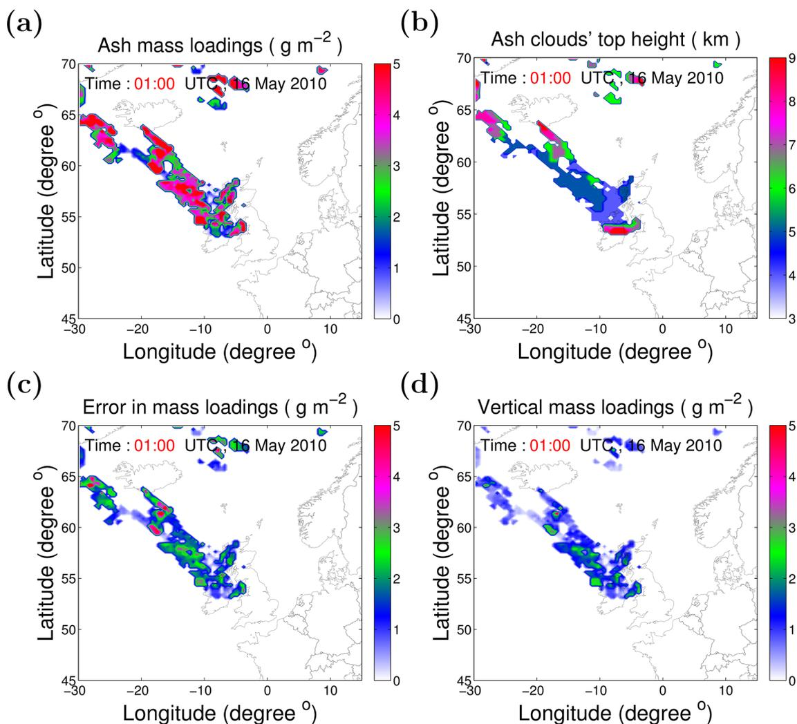
**Figure 1.** Available volcanic ash data from SEVIRI on 16 May 2010 at 01:00 UTC. Data are acquired from the European Space Agency (ESA) funded projects Volcanic Ash Strategic Initiative Team (VAST). (a) Ash mass loadings. Values at 0 mean no data. (b) Ash cloud top height. (c) Error in the retrieved ash mass loadings (a). (d) Ash mass loadings in the vertical direction, i.e.,  $M_v$  in Eq. (1).
