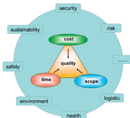
Figure D13: Representation of the dependency between scope, cost, speed and quality in terms of safety, risk, security etc. when realizing a system.
