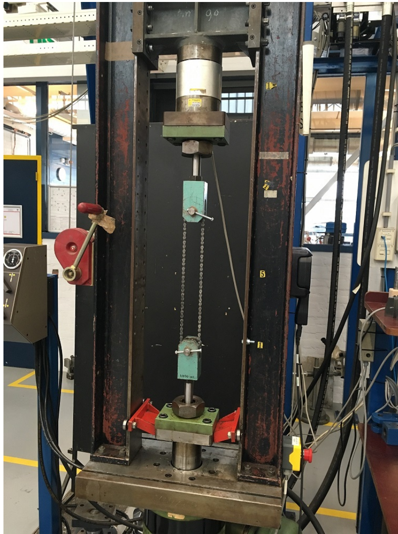
Fig. 5 Example bicycle chain in test machine.
