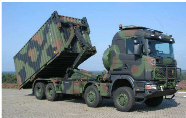
Figure 3.7: Figure of a truck equipped with a WLS, handling a container unit.
