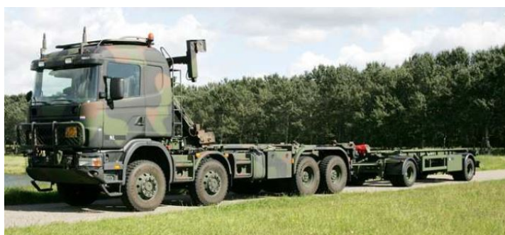
Figure 3.8: Figure of a truck equipped with WLS and TROPACO, used for heavy equipment transport.
