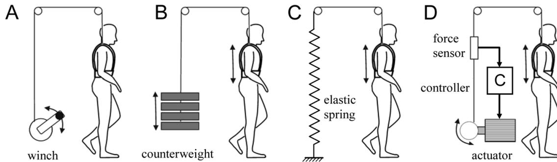
Figure 2.6: Body weight support systems concepts: (A) Static BWS (B) Passive dynamic BWS with adjustable counterweights (C) Elastic element-based passive dynamic BWS (D) Active dynamic BWS. Reprinted with permission from "A novel mechatronic body weight support system," by M. Frey et al., 2006, IEEE Transactions on Neural Systems and Rehabilitation Engineering. Copyright 2006 IEEE [27]
