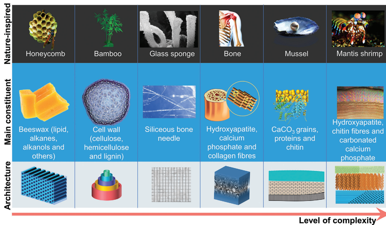
Figure 1. Typical architectures of nature-inspired. The compositions and unique structures across multiple length scales of biomaterials are key to achieving extraordinary mechanical properties and functionality. Different species of organisms have structures of varying complexity, largely depending on the living environment and functional requirements. Inspired by these biological structures, a range of bionic architectures have been designed from simple to complex.
