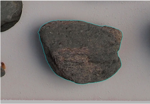
FIGURE 4 Outline of a pebble obtained from the application of the proposed method after calibration.
