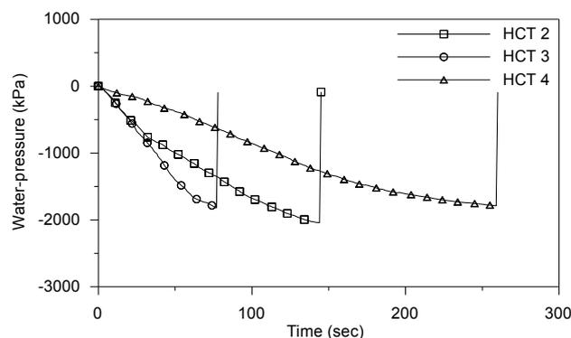
Figure 2. Response upon drying of UPPA tensiometers [6]
