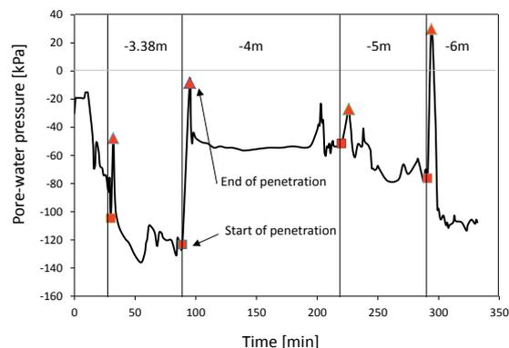
Figure 15. Field test of the penetrometer HCT
