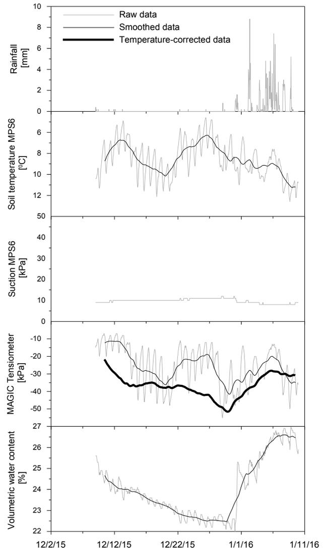
**Figure 7.** Response of the MAGIC HCT in the field and comparison with other sensors
