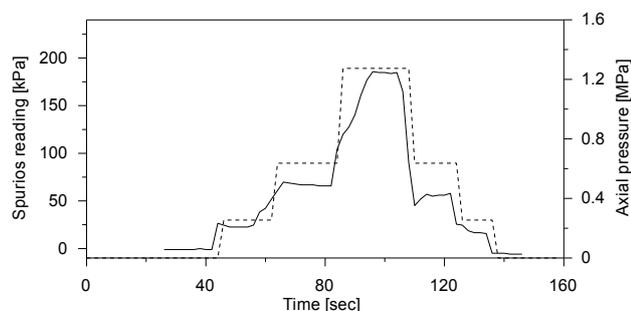
Figure 16. Mechanical effects on HCT tensiometer signal
