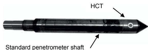
Figure 12. Prototype penetrometer shaft
