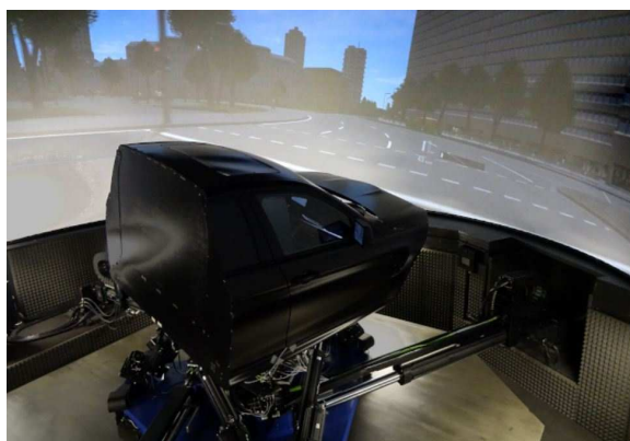
(a) The Driver-in-Motion simulator while moving during the experiment.
