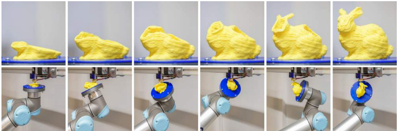
Figure 1: Our method enables support-free 3D printing of solid models. By exploiting all 6 degrees of freedom (translations, rotations) and depositing material along curved layers, we make support structures unnecessary in most cases. This increases further the flexibility offered by 3D printing, such as freeing designers from support constraints on complex parts.
