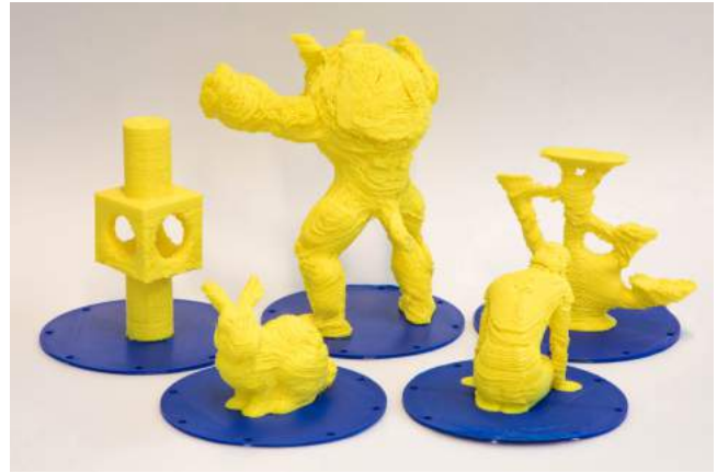
Figure 12: The 3D printing results of all examples shown in this paper.
