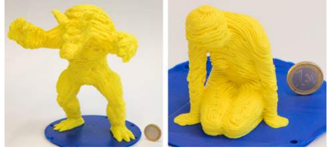
Figure 10: The results of our algorithm for 3D printing an Armadillo model and a Woman-Pully model by multi-axis motion.
