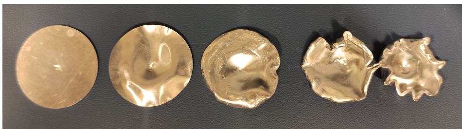
Figure 4.4: Flyer plates after being accelerated with increasing capacitor charge. The left most plate has not been accelerated.
