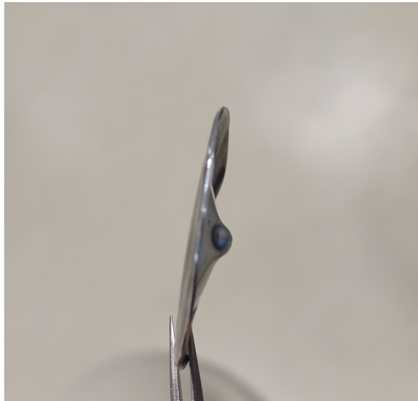
Figure 4.3: Flyer plate after acceleration: side view. The deformation due to the inertia of the projectile is clearly visible.
