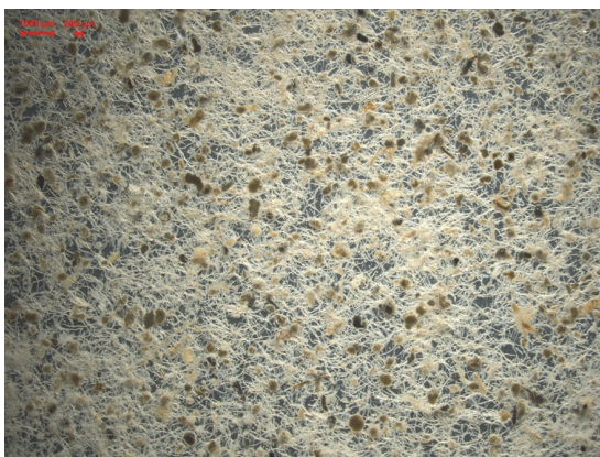
Figure 11.16 Image of sieved ( \geq 200\mu\text{m} ) excess sludge from a full-scale Nereda ® plant showing cellulose fibres meshed with pieces of granular sludge.
