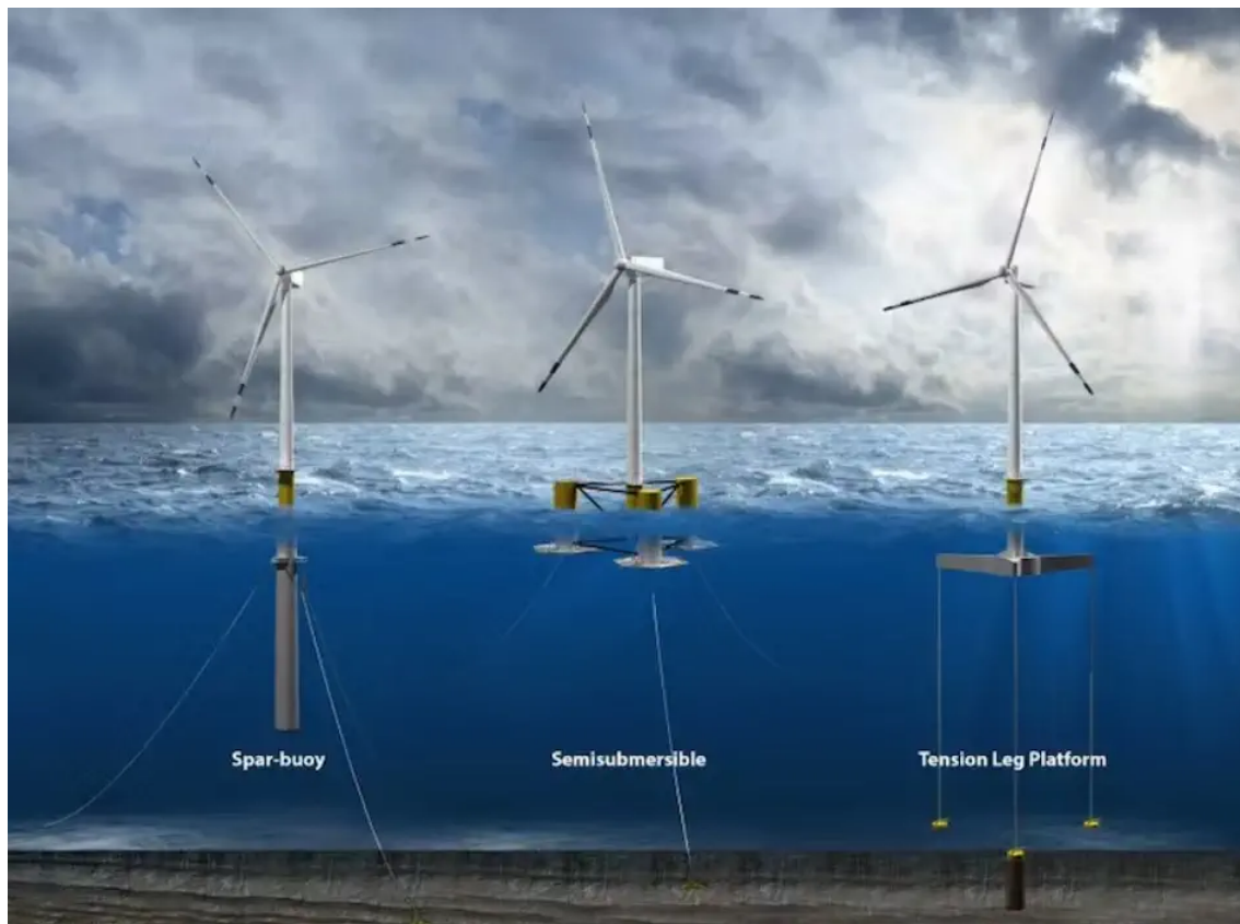
Figure 2.2: Type of wind turbines floaters, Spar Buoy, Semi-submersible, and Tension Leg Platform. Taken from [19].
