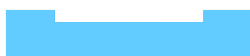
Figure C.1: PDMS bottom piece for disk and membrane curing. The slot is 180 \mu\text{m} deep and 6 mm wide (see appendix D). The dimensions in this image are not to scale.
