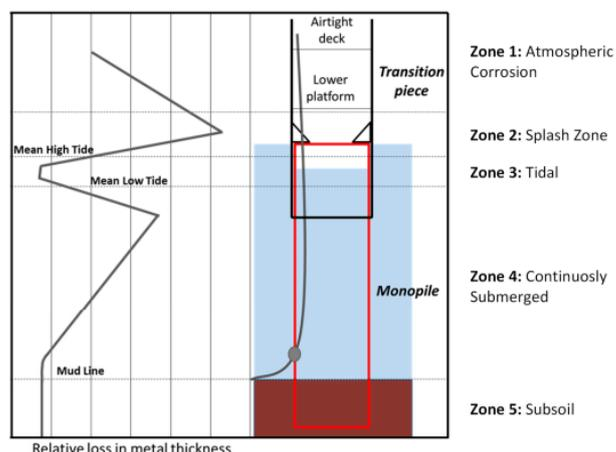
Figure 2.8: Suggested relative loss of metal thickness of unprotected steel on offshore wind turbine structure in seawater. Source: MDPI [49]
