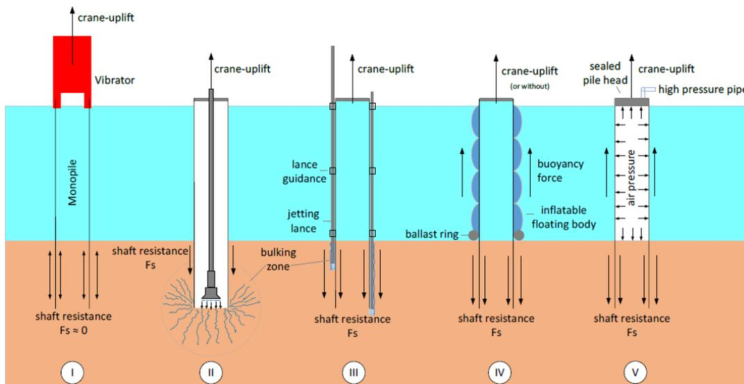
Figure 2.4: Possible offshore decommissioning techniques by Hinzmann [26]
