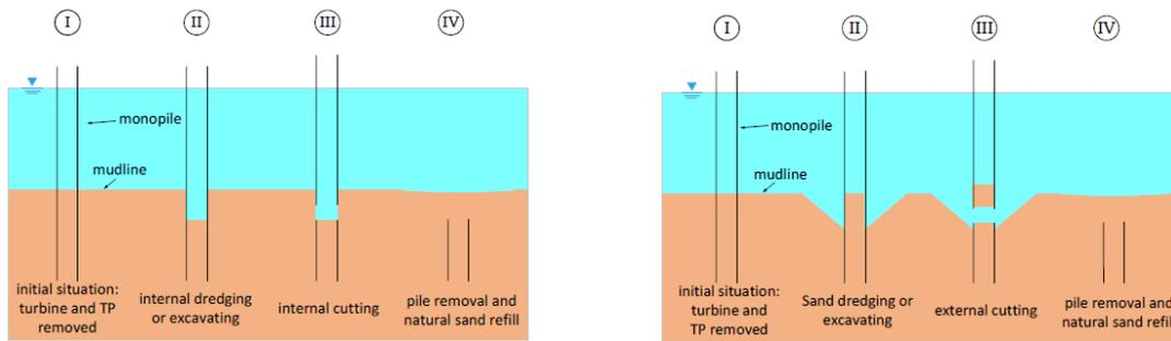
(a) Internal pile cutting. Source: Hinzmann [26]
