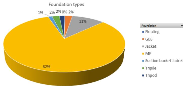
Figure 2.6: Foundation types of WTG's in the NSR
