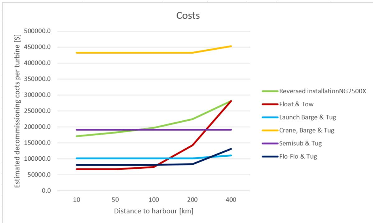
Figure 6.3: Costs per turbine per logistical configuration
