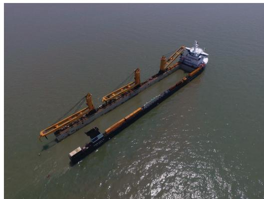
Figure 5.5: Submerged Flo-Flo vessel [24]
