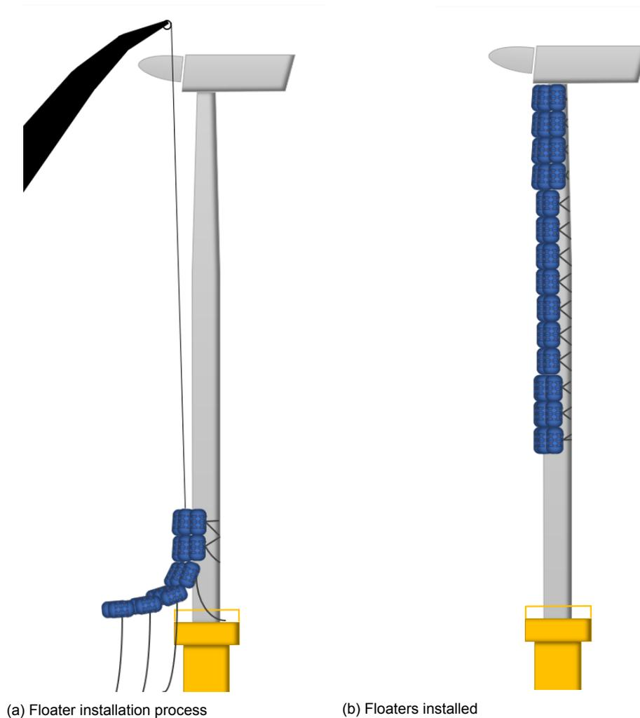
Figure 5.4: Floater installation
