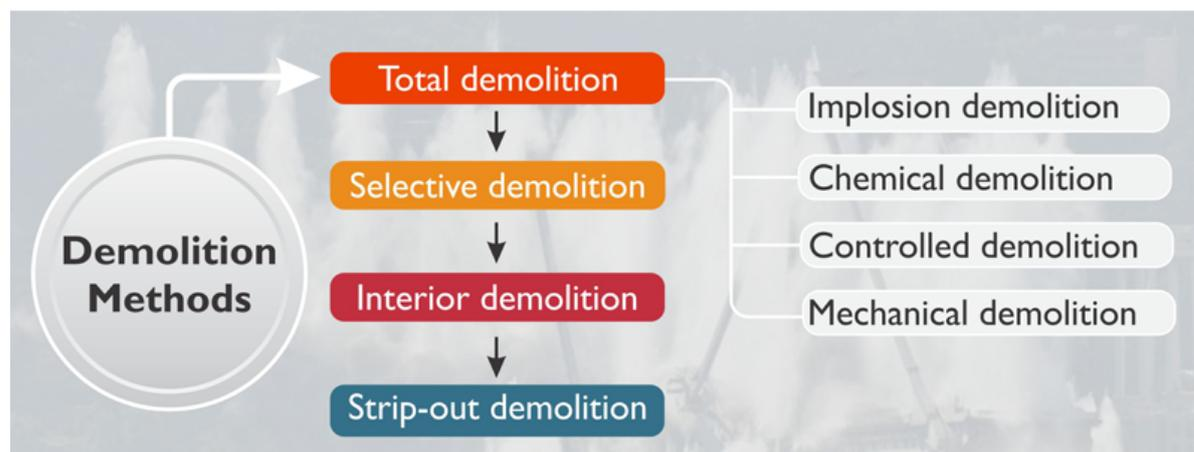
Figure 4.1: Demolition methods. Source: ConstroFacilitator [9]
