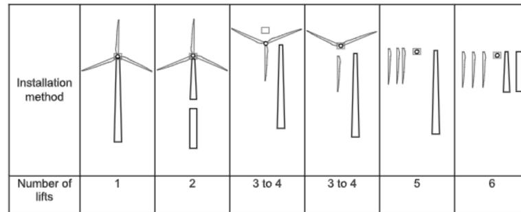
Figure 2.1: Installation methods offshore wind turbines. Source: Zhiyu Jiang [30]
