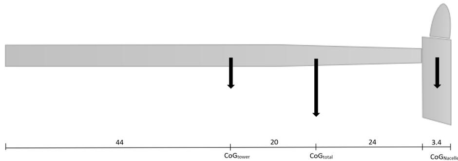
Figure 5.2: Centre of gravity 3.6MW turbine in [m]
