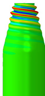
Figure 6.20: First buckling mode shape of the model including a radius of curvature of 380mm. Scaling factor is equal to 30.
