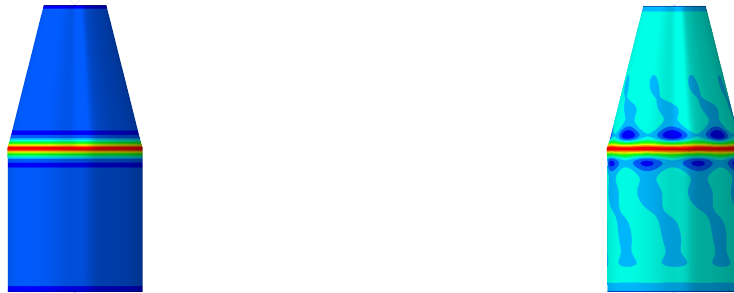
(a) Deformation shape prior to buckling. Taken at a displacement of 4.40 mm (b) Deformation shape at buckling load. Taken at a displacement of 3.95 mm with maximum U1 of 2.2 mm and minimum U1 of 0 mm.
