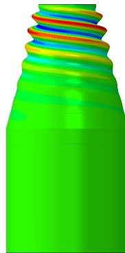
Figure 6.26: First mode shape of the reinforced cylindrical-conical shell. For generating this figure a scaling factor of 30 was employed.
