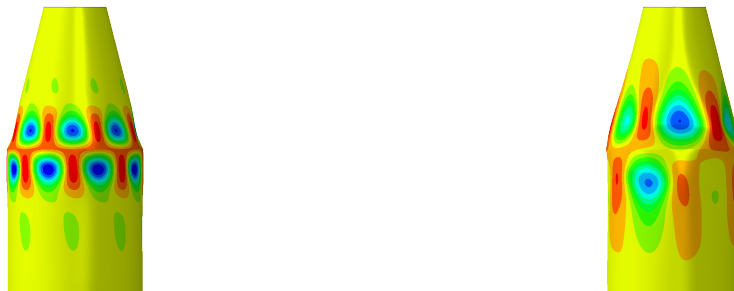
(c) Deformation shape right after buckling. Taken at a displacement of 3.96 mm with maximum U1 of 6.9 mm and minimum U1 of -14.5 mm. (d) Deformation shape in post buckling regime. Taken at a displacement of 8.31 mm with maximum U1 of 16.6 mm and minimum U1 of -42.7 mm.
