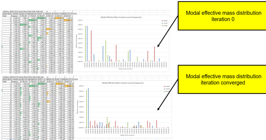
Figure 6.21: Model 1 solution 2 – modal effective mass fraction for the starting and converged iteration
