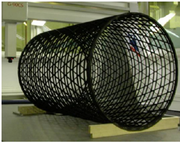
Figure 3.9: Central lattice composite structure for satellite architecture [34]
