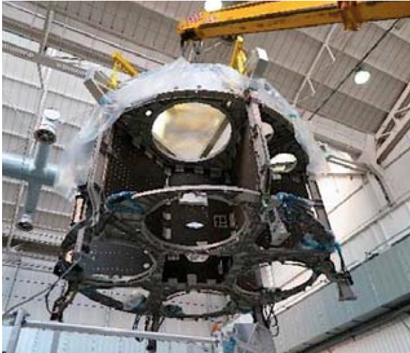
Figure 3.3: ESM main structure hardware [9]
