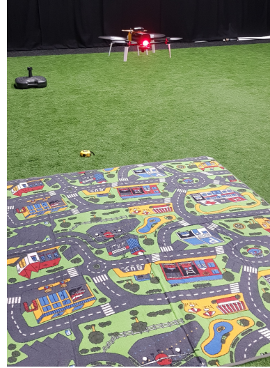
Figure 2: Parrot Bebop 2 quadrotor MAV equipped with SEEM1 Dynamic Vision Sensor.
