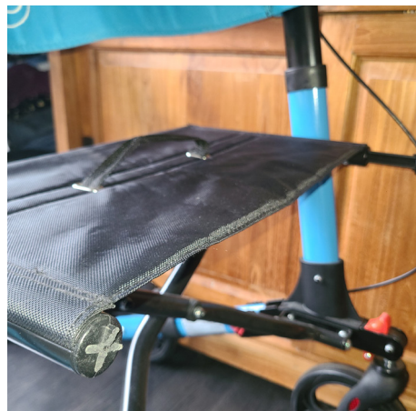
Figure 22 – Broken basket hook
