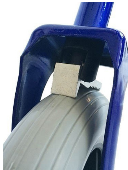
Figure 12 – Brake wear (rollatorwinkel.com, n.d.)
