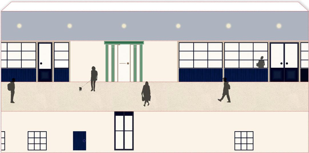
This is an unfolded fragment of the corridor, in front of the meeting room. The green portal of the meeting room remains as it is. For the rest of the floor a wooden structure is suggested, in that: a wooden panel is attached to it at the lower part, while in the rest of the height steel window frames on the same colour are suggested.
