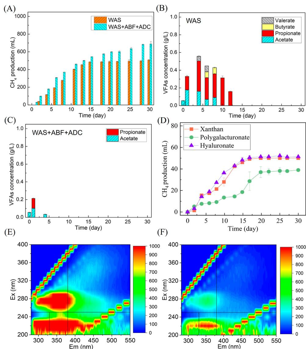
**Figure 3.** WAS fermentation with the addition of ABF. (A) Methane production; (B) VFA production in the WAS group; (C) VFA production in the WAS + ABF + ADC group; (D) methane production from three model compounds of uronic acids, and 3D-EEM fluorescence spectra of the TB-EPS layer in the WAS + ABF + ADC group on (E) days 0 and (F) 30.
