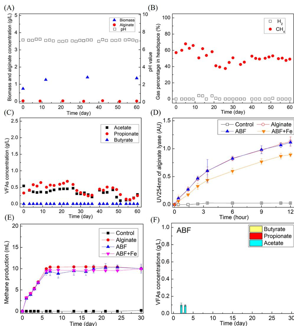
**Figure 2.** (A) pH values and biomass; (B) methane production; (C) VFA production in a mesophilic chemostat enriched with ADC; (D) extracellular alginate lyase activity; (E) methane production; (F) VFA accumulation from the prepared ABF.
