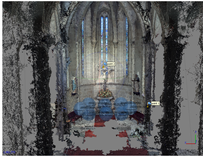
Figure 5.4: Point cloud generated from panoramic images using Agisoft Photoscan .
