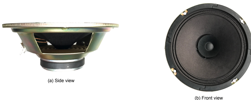
Figure 1.1: Example of a moving-coil electrodynamic loudspeaker.
