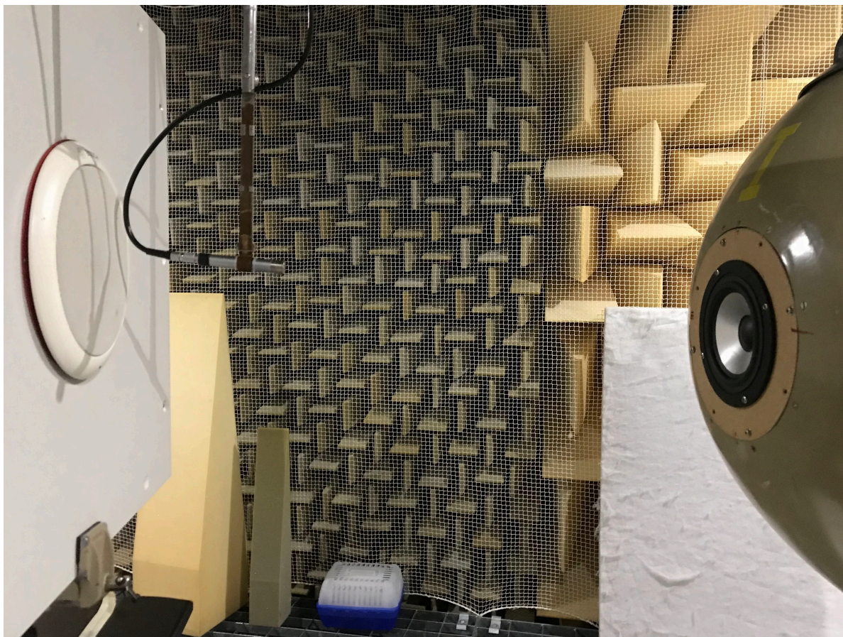
Figure 5.2: A close-up of the setup used for measuring the recording response of loudspeakers. The height of the loudspeaker did not match that of the microphone and the device under test (DUT). Also the microphone position is not ideal, as it should be right next to the DUT. These non-idealities should be compensated for in the measurements.
