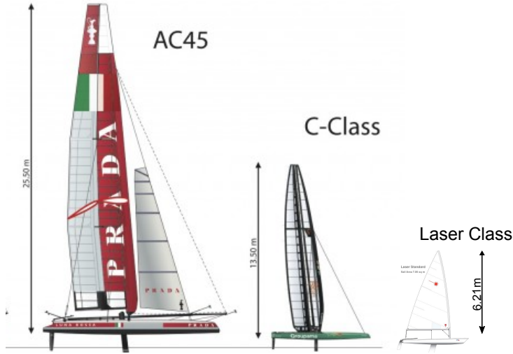
Figure 4.5: Mast Height Comparison between two yachts models AC45 and C-Class versus the Laser Olympic Class, side view. [41].
