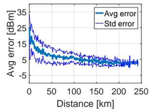
Figure 2: Error between Friis model and measurements.
