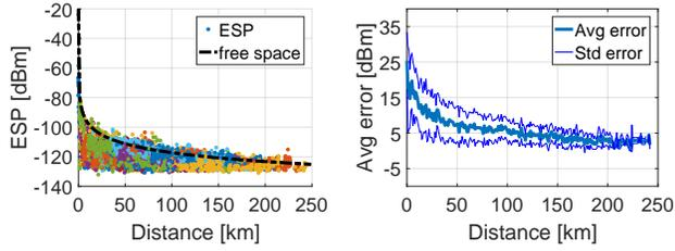
Figure 1: ESP vs. distance for all gateways.
