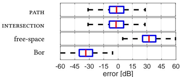
**Figure 18: Overall estimation error (median, 25<sup>th</sup> and 75<sup>th</sup> percentile) on samples with devices  $\leq 2\text{m}$  height: PATH, INTERSECTION, free-space and Bor.**
