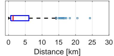
Figure 4: Variation of communication ranges for LoRa links.
