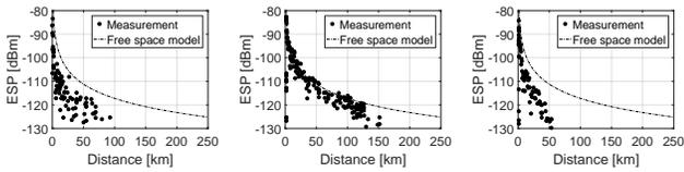
Figure 3: ESP vs. distance for selected gateways.
