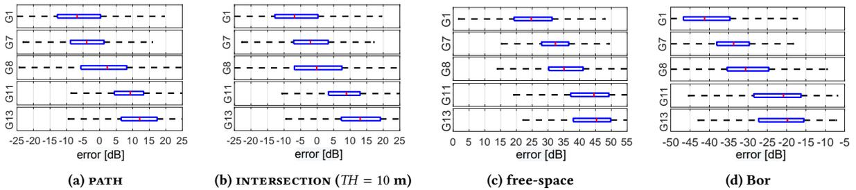
**Figure 17: Per-gateway statistics of the estimation error (median value, 25<sup>th</sup> and 75<sup>th</sup> percentile) for PATH, INTERSECTION, as well as free-space and Bor models, for end-devices with height  $\leq 2\text{m}$ .**
