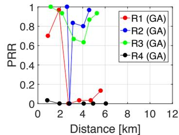
Figure 7: PRR vs. distance for gateway GA.
