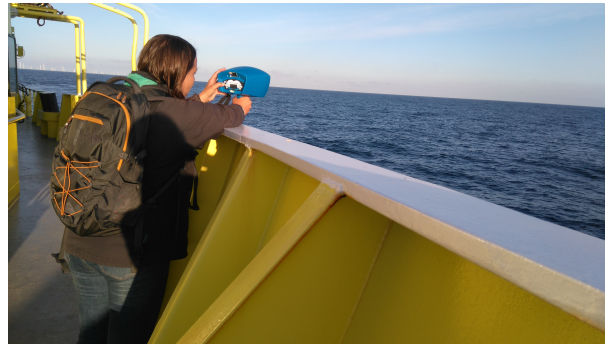
Figure 7.2: Picture of the WISP. The WISP uses 3 spectrometers to observe the solar irradiance, the water-leaving radiance and the sky radiance. From these measurements chlorophyll and TSM products can be determined.
