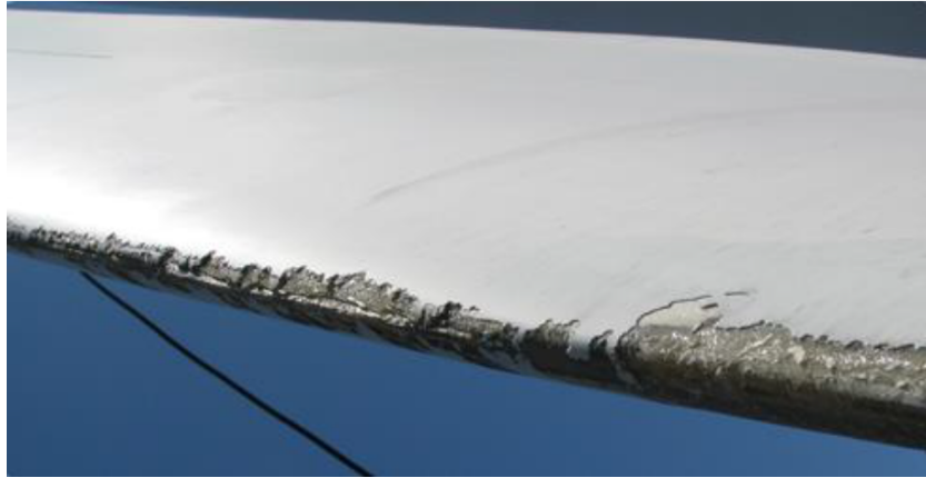
Figure 1.2: An example of leading edge erosion. Source: [24]
