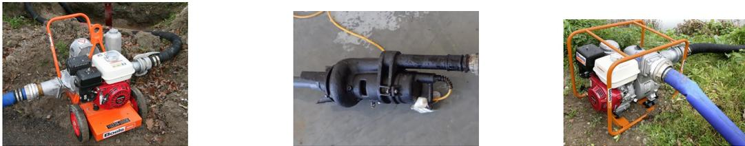
Figure 5.2: Three different tested pumps: Diaphragm (4.5m<sup>3</sup>/h), Hidrostal(30m<sup>3</sup>/h) and centrifugal(30m<sup>3</sup>/h)
