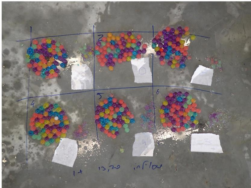
Figure 5.4: Example of the damage to hydrogel balls following pumping for six tests. The balls are soaked over night with the same duration and therefore have the same dimensions and properties.
