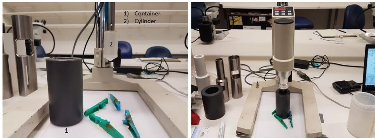
Figure 3.3: Setup of the Couette-rheometer (type: HAAKE VT550) to investigate the strength threshold of coral embryos and larvae.
