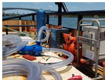
Figure 1.2: Hidrostal(blue) and Diaphragm pump(red)
