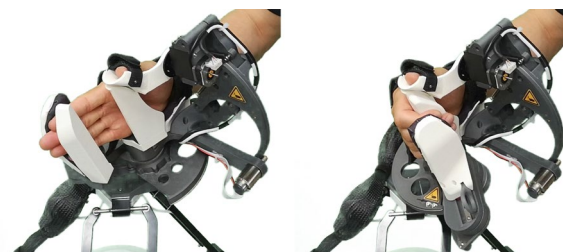
Fig. 2 Collective finger flexion and extension movements
