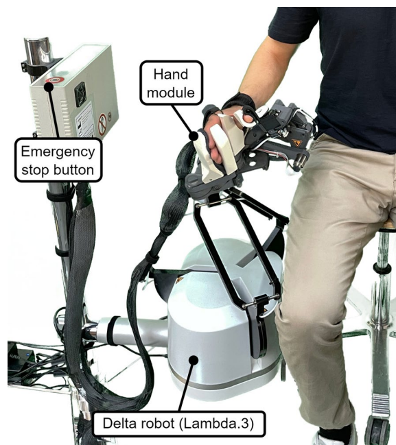
Fig. 1 The Lambda.3+ haptic device consists of a delta robot (Lambda.3) and a custom hand module with hand-size-specific exchangeable handles. The user is ready to grasp a virtual object with extended fingers and abducted thumb
