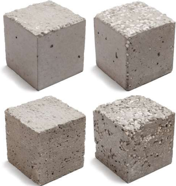
figure 39: Polystyrene and concrete
