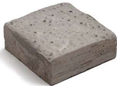
figure 49: Concrete and optic fibers
