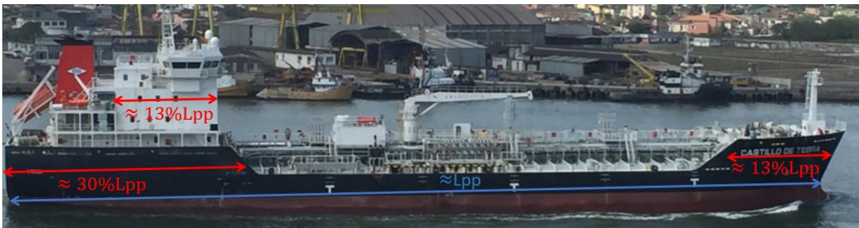
Figure 9: Side view of the ship with size estimations of the superstructures and deckhouse based on the L_{pp} ( https://www.shipspotting.com/photos/2734272?navList=moreOfThisShip&imo=9753636&lid=2738636 ).
