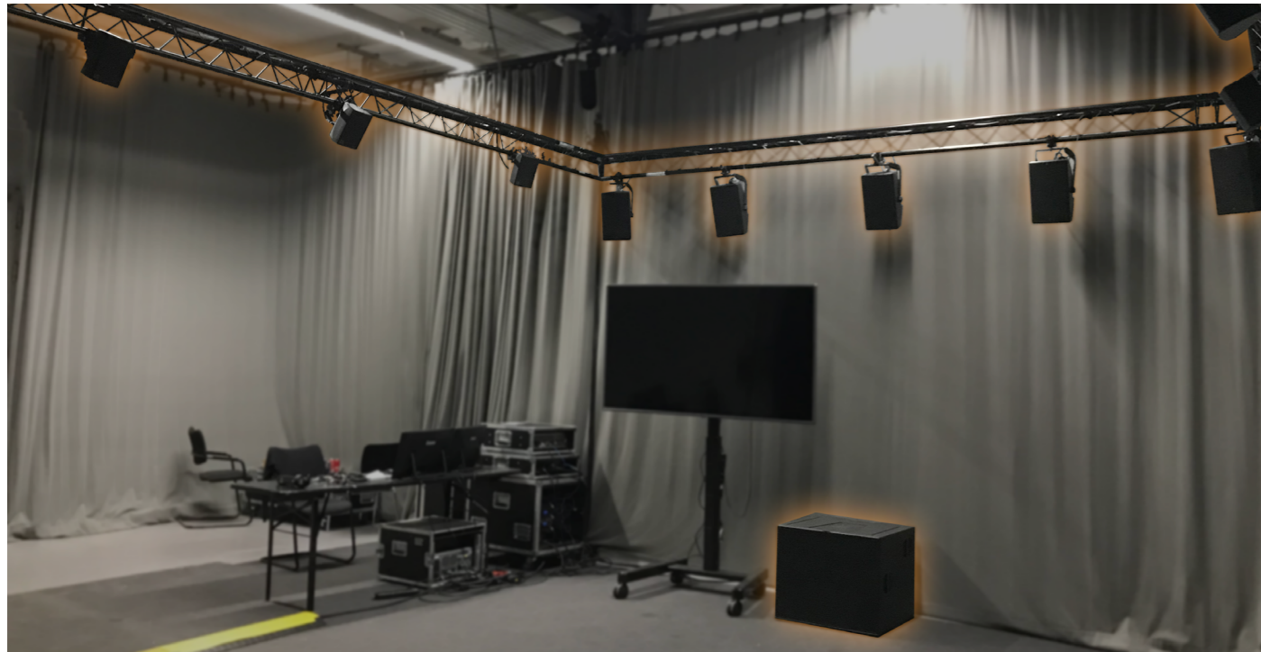
Figure 1: an immersive loudspeaker setup with loudspeakers surrounding the audience, highlighted in orange.
