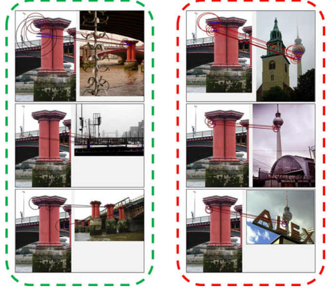
Fig. 7. Illustration of the initial correspondence set between the query image and the photos in two different locations with the color intensity from black to red representing the increase of the strength of the initial matching score. The left photo set is from the same location as the query image.
