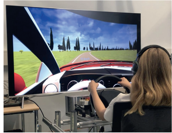
FIGURE 2: The experimental environment with a participant driving in the fixed-based simulator. The digital speedometer can be seen in light blue font, just above the bonnet.
