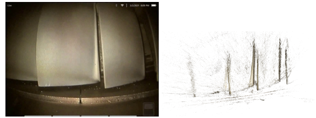
Figure 6: Video 2 comparison of reference video and GT dense model. Blades can be clearly recognised.
