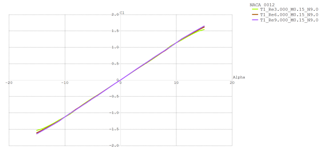
Figure 5.3: NACA0012 C_{L\alpha} curve as generated by XFLR5.
