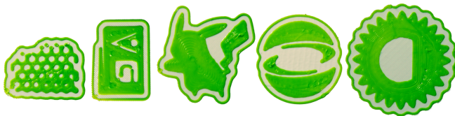
Fig. 19. Photographs of prints obtained on the Ultimaker S5. Because S^0 is 2\gamma -fat rather than \gamma -fat, a large part of the hexagonal grid is missing; See Figure 15. The second print from the left is 2/3 the scale of the one on Figure 18. This renders the hook \gamma less than 2\gamma -fat in the stem, so that a small part of it has been removed.
