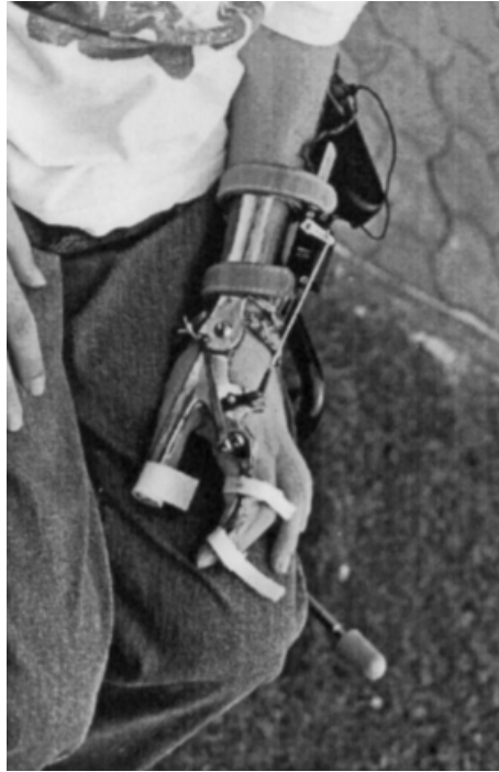
Figure 8: An electrical hand orthosis attached with Velcro. Adapted from Pfurtscheller et al. (2000)
