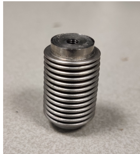
Figure 5. The bellows. On top the bellows cap is visible with the M3 thread.
