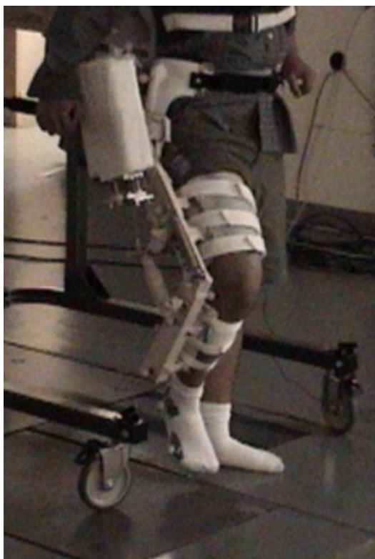
Figure 7: A leg orthosis attached with Velcro. Adapted from Banala et al. (2006)
