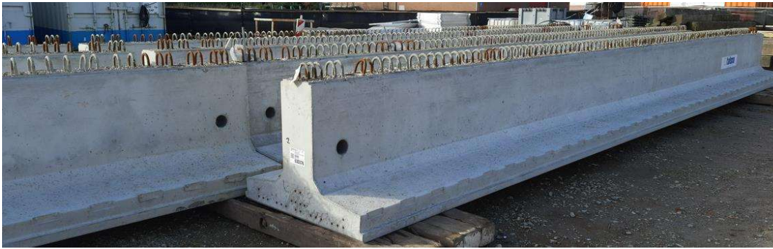
Fig. 4 (a) Specimen details (all dimensions are in mm) (b) Specimens before connection (note the location of the strands and the hairpins)
