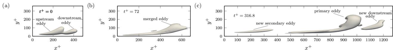
Figure 1: Iso-contours of swirling strength squared (10% of maximum) at time  $t^+ = 0, 72$  and  $316.8$  for the two-eddy case with stream-wise separation  $\Delta x^+ = 118$  (side view). Two eddies in (a) merge to form a single stronger eddy in (b). Merged eddy further auto-generates as shown in (c).  $x^+$  and  $y^+$  represent stream-wise and wall-normal directions, respectively, normalized by wall units.
