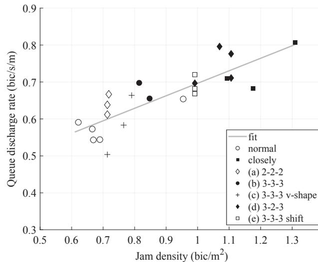
Fig. 7. Jam density and the queue discharge rate.
