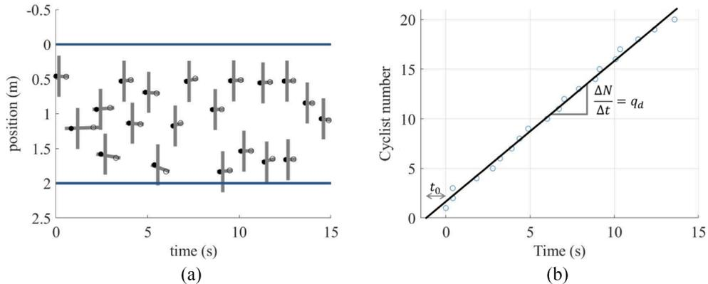
**Fig. 5.** The digitized version of 4b showing the lateral position and passing time of all bikes (a). The front wheel is indicated with the filled dot, the rear wheels with the open dot. (b) shows an example of the regression analysis to obtain the queue discharge rate.
