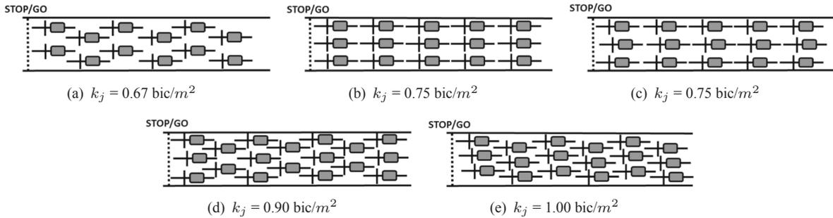
Fig. 3. Tested queue configuration with theoretical jam densities.
